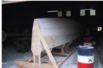
Hull is faired below waterline before turning
