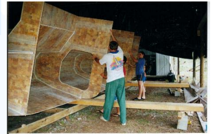
Turning the first hull
