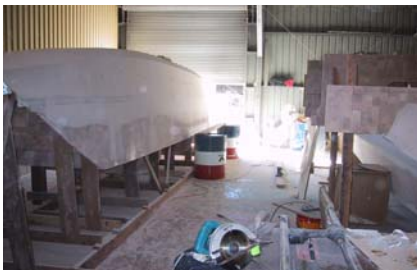
One hull up and the second hull ready to turn over.
