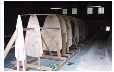
Bulkheads up and ready for hull panels
