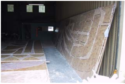
Pre-cut pre-glassed panels with peelply.
