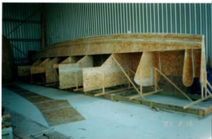
Hull panels are fitted and taped
