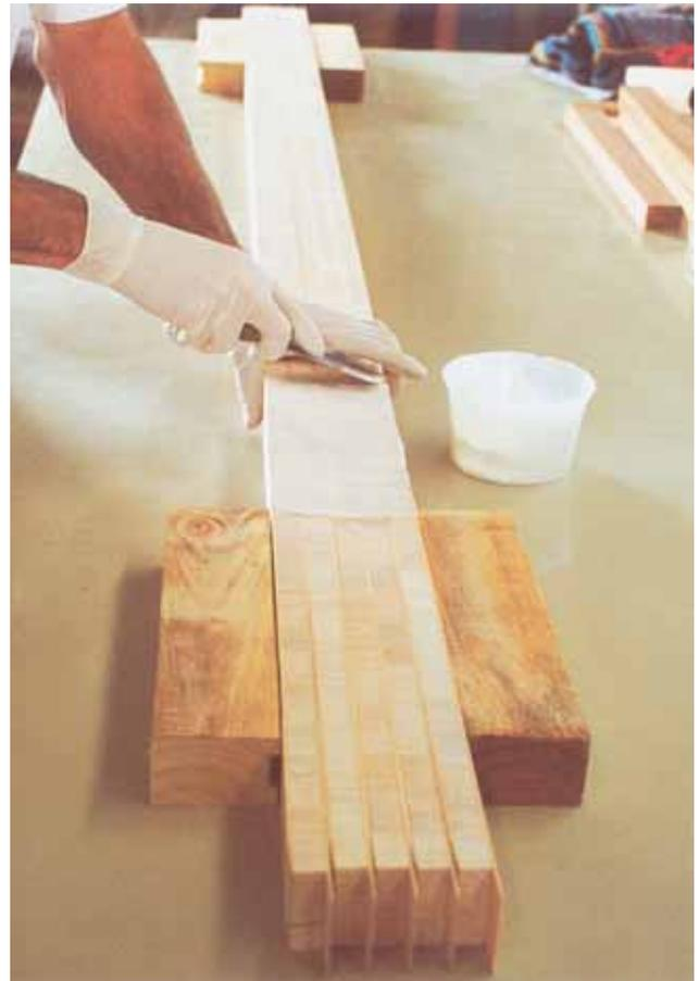
After removing each bundle of strip planks scrape any excess epoxy/filler from the jig before it cures. It is important to keep the jig clean, especially the two top edges that guide the trowel while smoothing the correct thickness of epoxy/filler over the strip planks. If enough epoxy cures on the jig to reduce its effectiveness, remove and replace the layer of protective plastic packaging tape.
