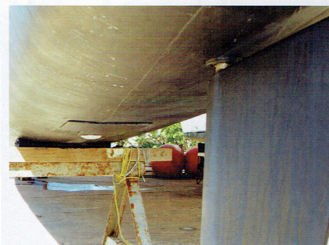
Motor up with plate closing hull.
