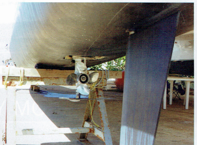
Motor down showing prop position in relation to the rudder.
