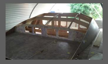
The two hulls are built separately and upside down over bulkheads which are set in place on a strongback. The strongback material is not supplied in the kit.
