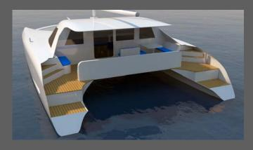
The cockpit is big and safe with full shade cover and plenty of seating and your option of steering position, single wheel on the bulkhead or twin sports wheels outboard, and the option of an internal helm station for colder climates. Cockpit seating is generous with sill height set at seat level allowing better volume in the aft cabins and more wave protection for ocean sailing and those tricky bar crossings. Not to mention it just might help keep those crocs out of the cockpit up north!
