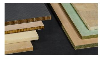
cubic metre) in compression. Foam is stronger than honeycomb type cores, both the paper and the plastic.
