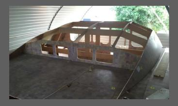
over bulkheads which are set in place on a strongback. The strongback material is not supplied in the kit.
