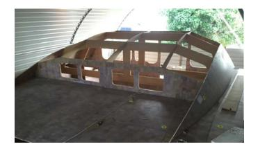
over bulkheads which are set in place on a strongback. The strongback material is not supplied in the kit.
