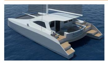
carbon where appropriate. The Arrow 1280-S will be offered with a carbon fore beam option, pricing will be available in due course. A pre-cut kit will be available for the 1280-S and her construction follows the Arrow Series and features 100% flat panels, reducing build time.
